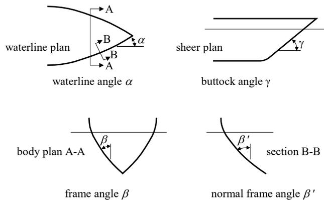
Note:  $\beta'$  = normal frame angle at upper ice waterline, degrees
