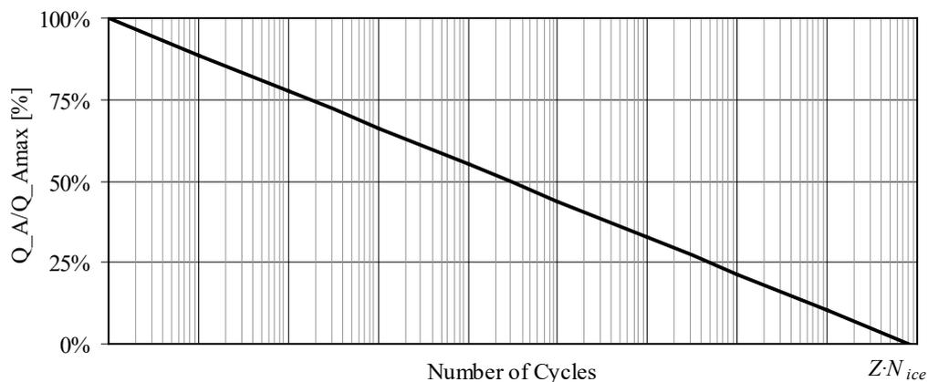
$Q_{Amax}$  is the average response torque shown in 6-1-3/Figure 2, calculated by means of transient torsional vibration analysis.
