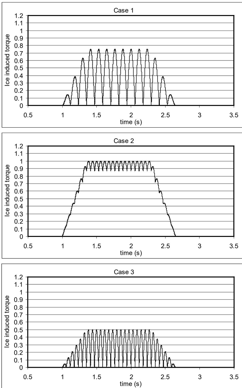
9.11.2 Response Torque in the Propulsion System (1 July 2019)
