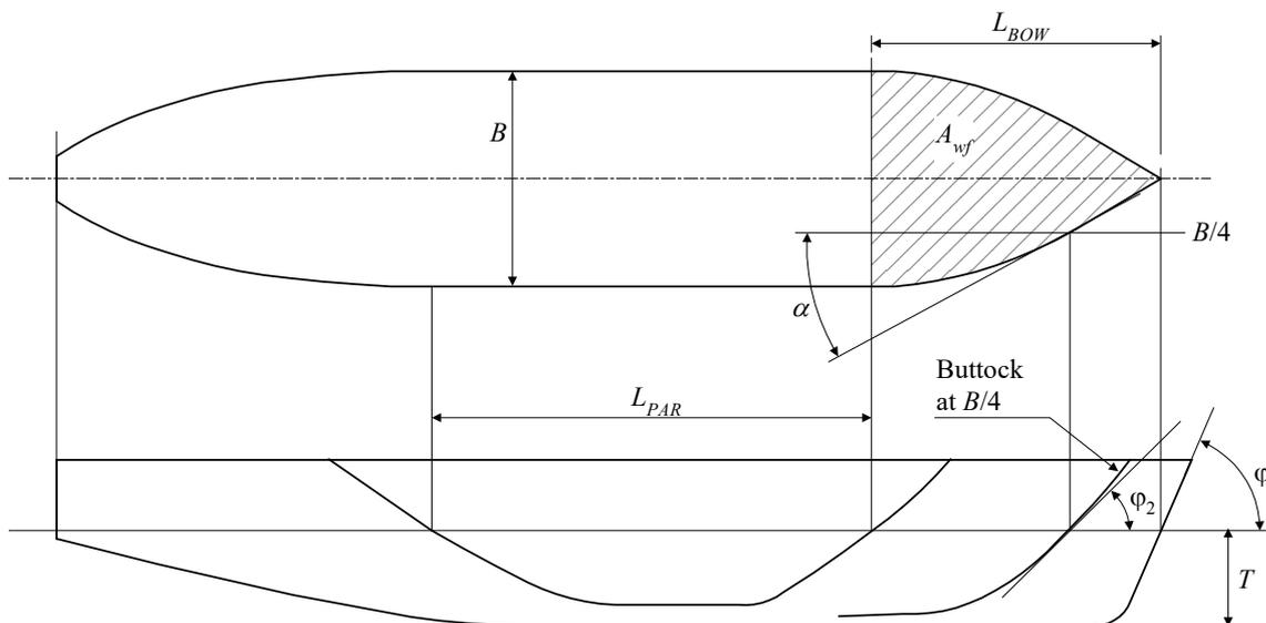
For a vessel with a bulbous bow,  $\varphi_1$  is to be taken as  $90^\circ$ .
