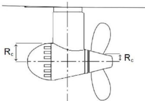
For impacts on non-hemispherical areas, such as the impact on the nozzle, the equivalent impact sphere radius must be estimated using the equation below.
