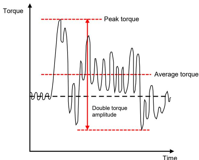
*Note:* For transient torsional vibration analysis (time domain), the model should include the ice excitation at the propeller, the mean torque values provided by the prime mover and the hydrodynamic mean torque produced by the propeller as well as any other relevant excitations. The aim of torsional vibration calculations is to estimate the torsional loads for individual shaft line components in order to determine scantlings for safe operation.
