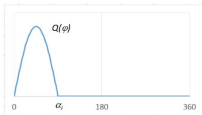
The total ice torque is obtained by summing the torque of single blades, while taking account of the phase shift  $360 \text{ deg}/Z$ , see 6-1-6/Figure 10 or 6-1-6/Figure 11. At the beginning and end of the milling sequence (within the calculated duration) linear ramp functions shall be used to increase  $C_q$  to its maximum value within one propeller revolution and vice versa to decrease it to zero (see the examples of different  $Z$  numbers in 6-1-6/Figure 10 or 6-1-6/Figure 11).
