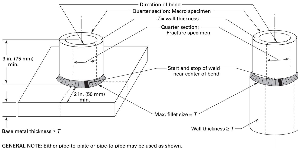
GENERAL NOTE: Either pipe-to-plate or pipe-to-pipe may be used as shown.
