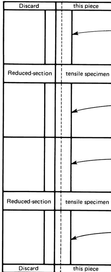
Longitudinal first surface bend specimen
