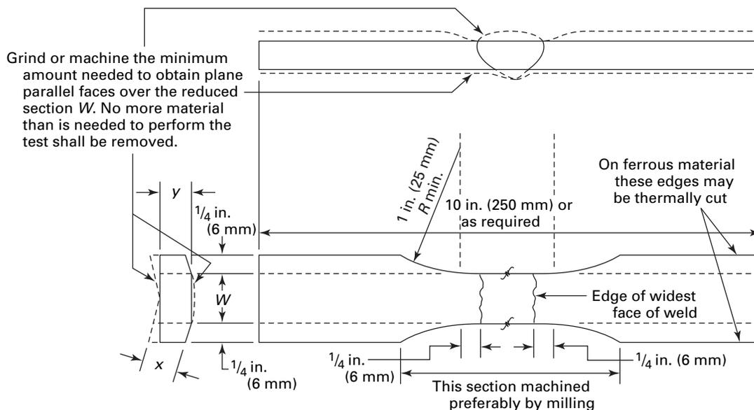
QW-462.1(c) TENSION — REDUCED SECTION ALTERNATE FOR PIPE
