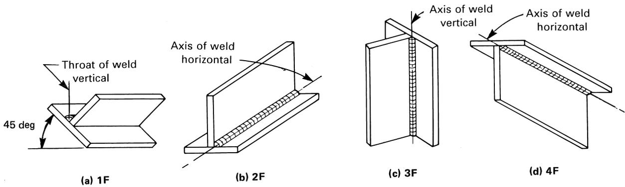
QW-461.6 FILLET WELDS IN PIPE — TEST POSITIONS
