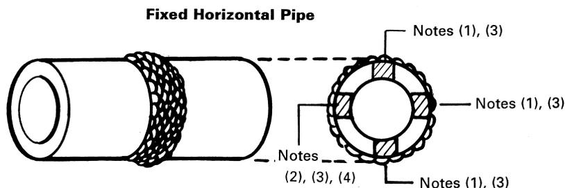
Test Specimen Location for 5G Overlay Qualification
