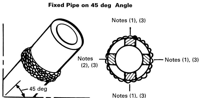
Test Specimen Location for 6G Overlay Qualification
