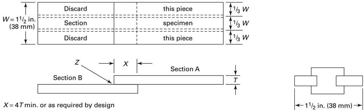
GENERAL NOTE: Specimen shall be brazed from the side marked Z.
