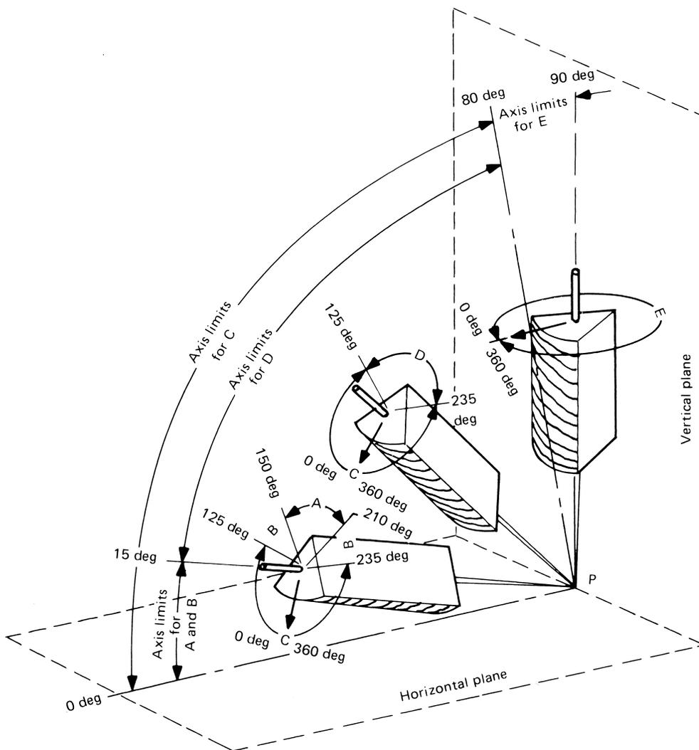
QW-461.3 GROOVE WELDS IN PLATE — TEST POSITIONS
