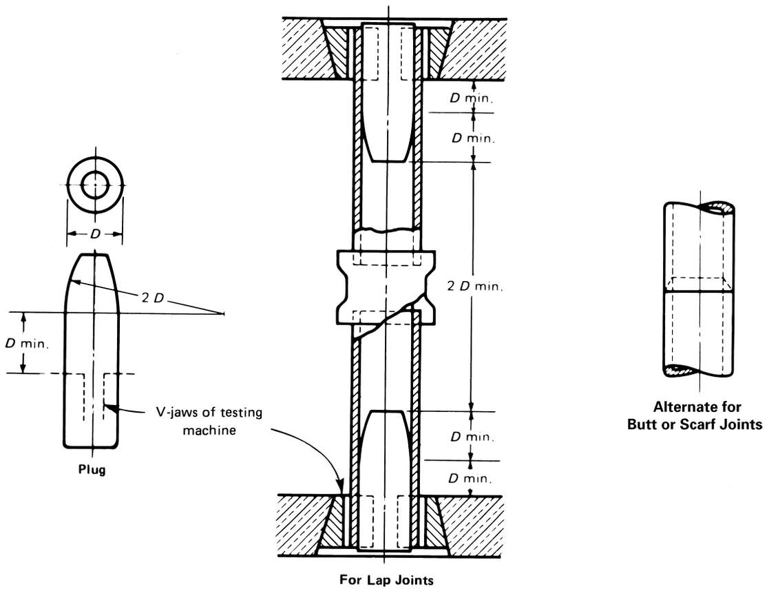
QB-462.1(f) SUPPORT FIXTURE FOR REDUCED-SECTION TENSION SPECIMENS
