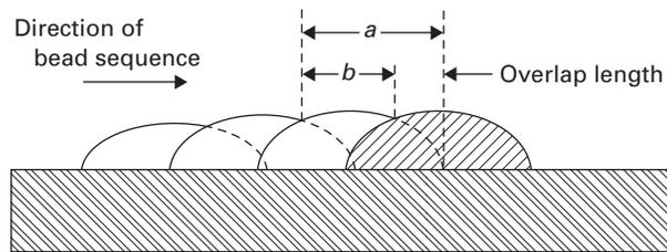
GENERAL NOTE: Measurement of bead overlap – % overlap length =  $(a-b)/a \times 100\%$ . In this figure, the shaded bead overlaps previous bead by 30% to 40%. The distance  $a$  is measured before the next bead is deposited.
