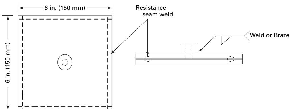
QW-462.7.2 SEAM WELD SECTION SPECIMEN REMOVAL
