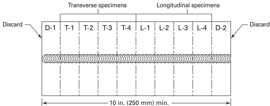
GENERAL NOTE: Mark the coupon into ten equal length specimens, label one end of the coupon D-1 the other end D-2. Cut the 10 in. (250 mm) coupon (transverse to the weld length) into pieces 5 in. (125 mm) long each.
