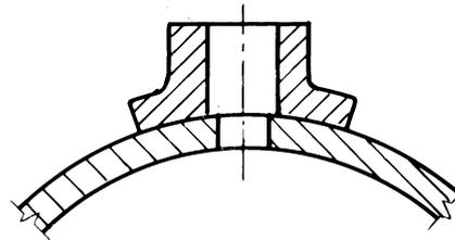
(c) Typical Saddle Joint Sectioned
