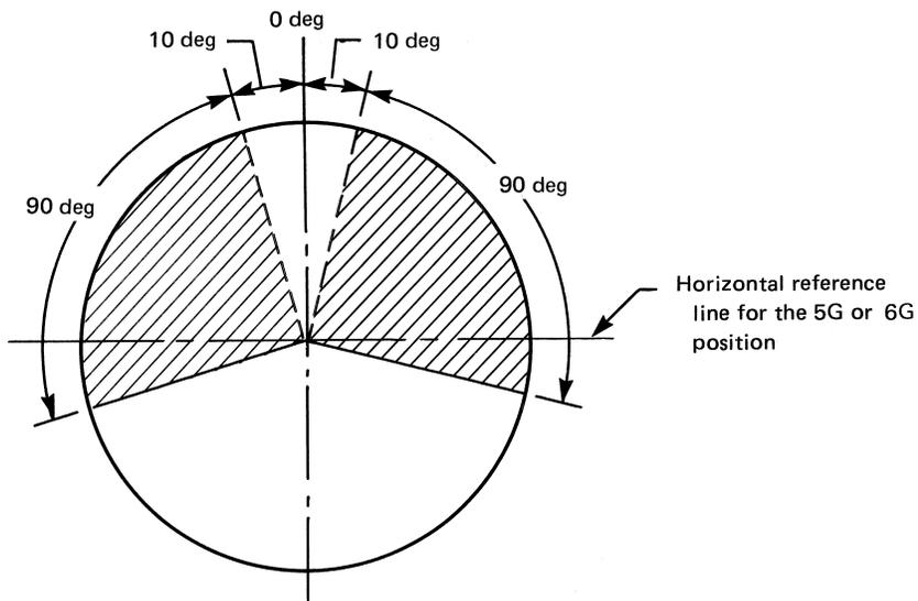
QW-463.2(a) PLATES — LESS THAN  $\frac{3}{4}$  in. (19 mm) THICKNESS PERFORMANCE QUALIFICATION
