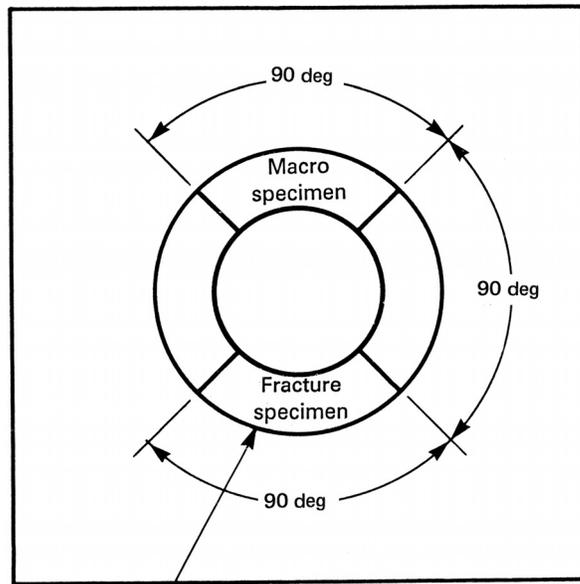
Fracture specimen to be removed from lower 90 deg section in position 5F
