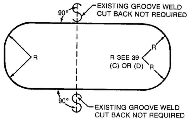
(F) ACCESS OR INSERT CROSSING EXISTING GROOVE WELD
