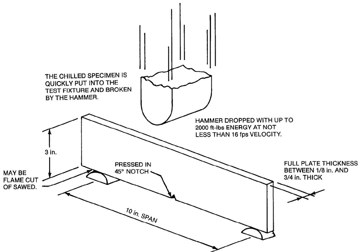
Figure D-7—Drop Weight Tear Test (ASTM E436)
