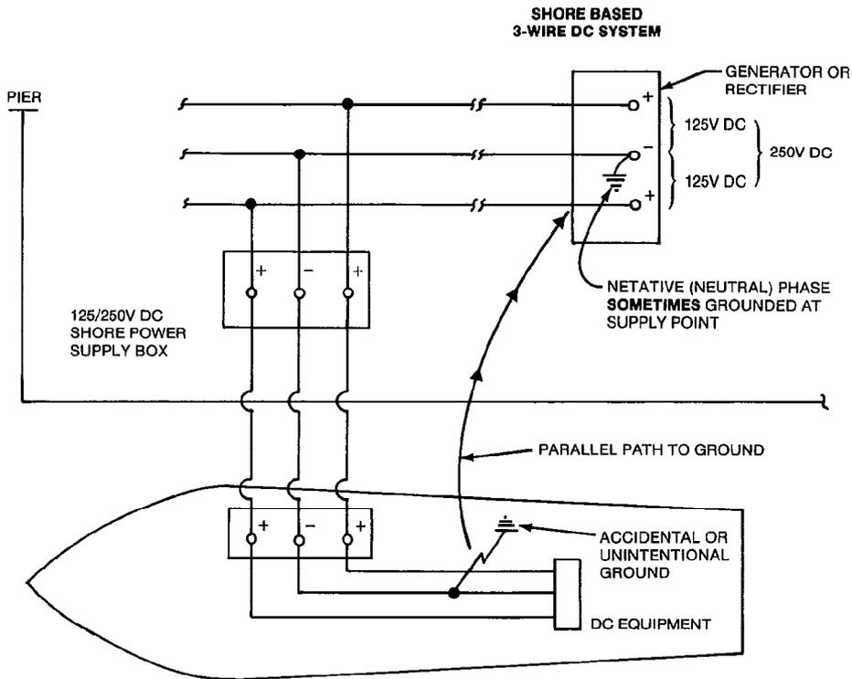
**Figure 52—Potential Source of Direct Currents Causing Corrosion Due to Accidental or Unintentional Ground on Vessel**
