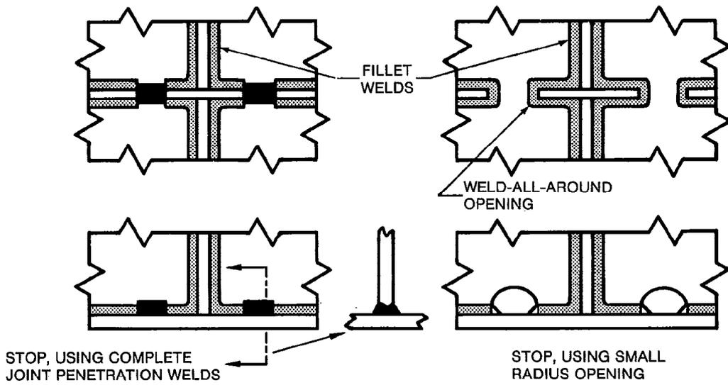
Figure 25—Welded Water- or Oil-Stops at Intersecting Members
