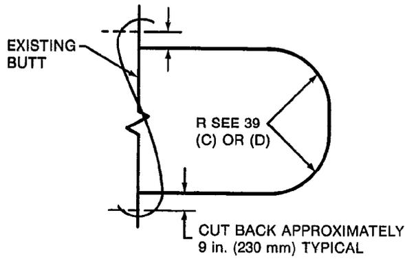
(E) ACCESS OR INSERT LANDING ON EXISTING BUTT
