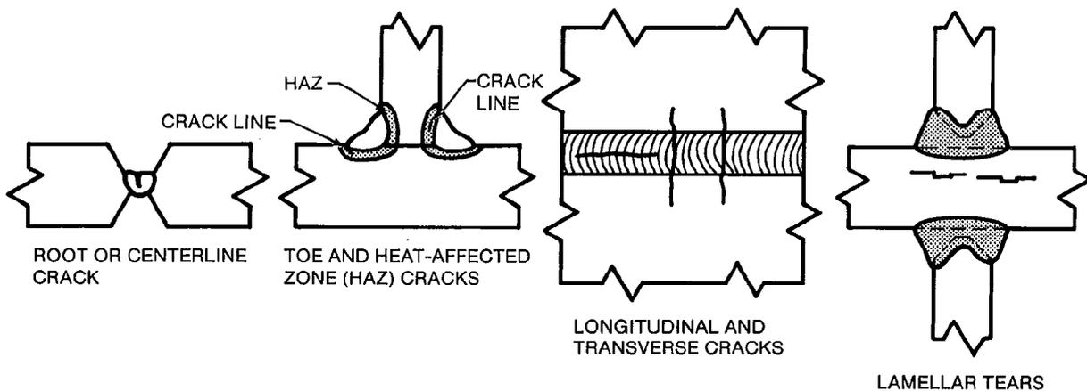
Figure 49—Typical Weldment Cracks
