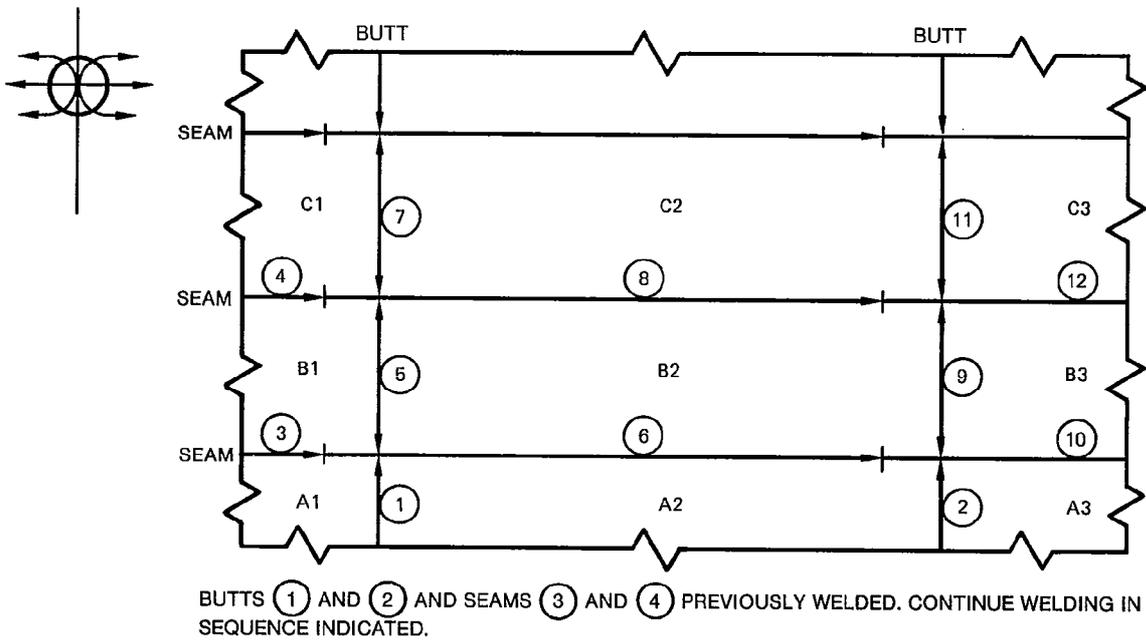
BUTTS ① AND ② AND SEAMS ③ AND ④ PREVIOUSLY WELDED. CONTINUE WELDING IN SEQUENCE INDICATED.
