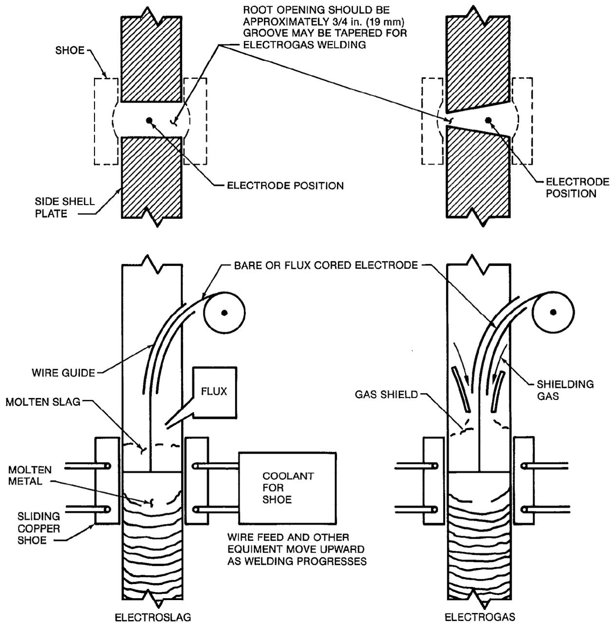
Figure 9—Vertical Electroslag and Electrogas Welding
