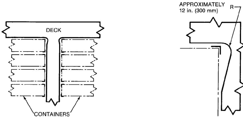
Figure 17—Typical Hatch Corner in Way of Container Guides on Container Ship
