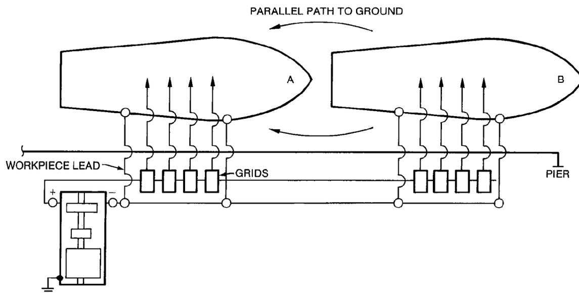
NOTE: WHEN TWO SHIPS ARE CONNECTED TO THE SAME GENERATOR OR RECTIFIER, THE RESISTANCE OF THE NEGATIVE RETURN BETWEEN THE SHIPS CANNOT BE MADE LOW IN COMPARISON WITH THE RESISTANCE THROUGH THE WATER. SOME OF THE CURRENT USED ON SHIP B FLOWS THROUGH THE WATER, CORRODING METAL OFF SHIP B AND POSSIBLY BLISTERING PAINT ON SHIP A.
