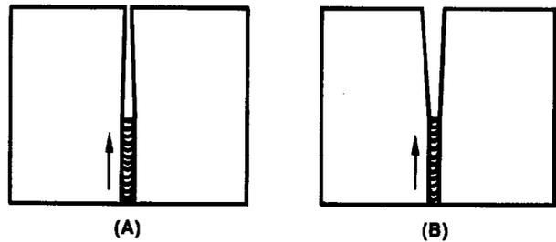
Figure 43—Angular Distortion Tendencies in Making Groove Welds
