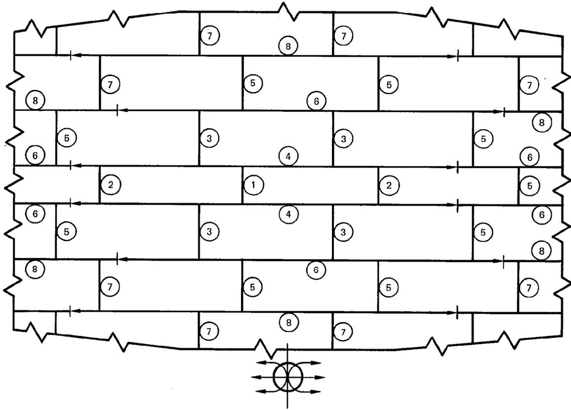
Figure 34—Typical Welding Sequence For Plate Butts and Seams Where Butts are Staggered
