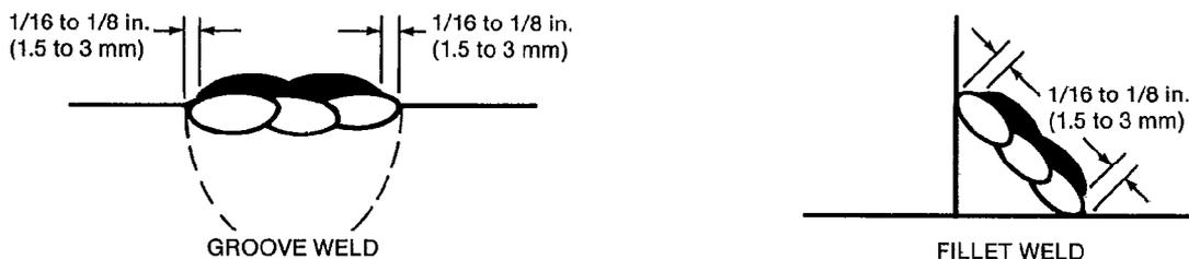
NOTE: TEMPERING BASES, SHOWN IN BLACK, SHOULD BE DEPOSITED APPROXIMATELY 1/16 to 1/8 in. (1.6 to 3 mm) FROM THE BASE MATERIAL
