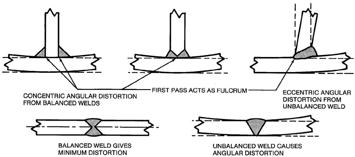
Figure 41—Typical Distortion of Welded Joints
