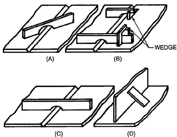
**Figure 29—Typical Strongbacks**
