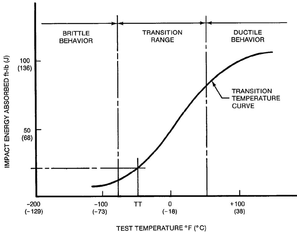
NOTE: TRANSITION TEMPERATURE (TT) IS DEFINED AS THE TEMPERATURE AT WHICH THE CURVE CROSSES A SPECIFIED ENERGY VALUE.
