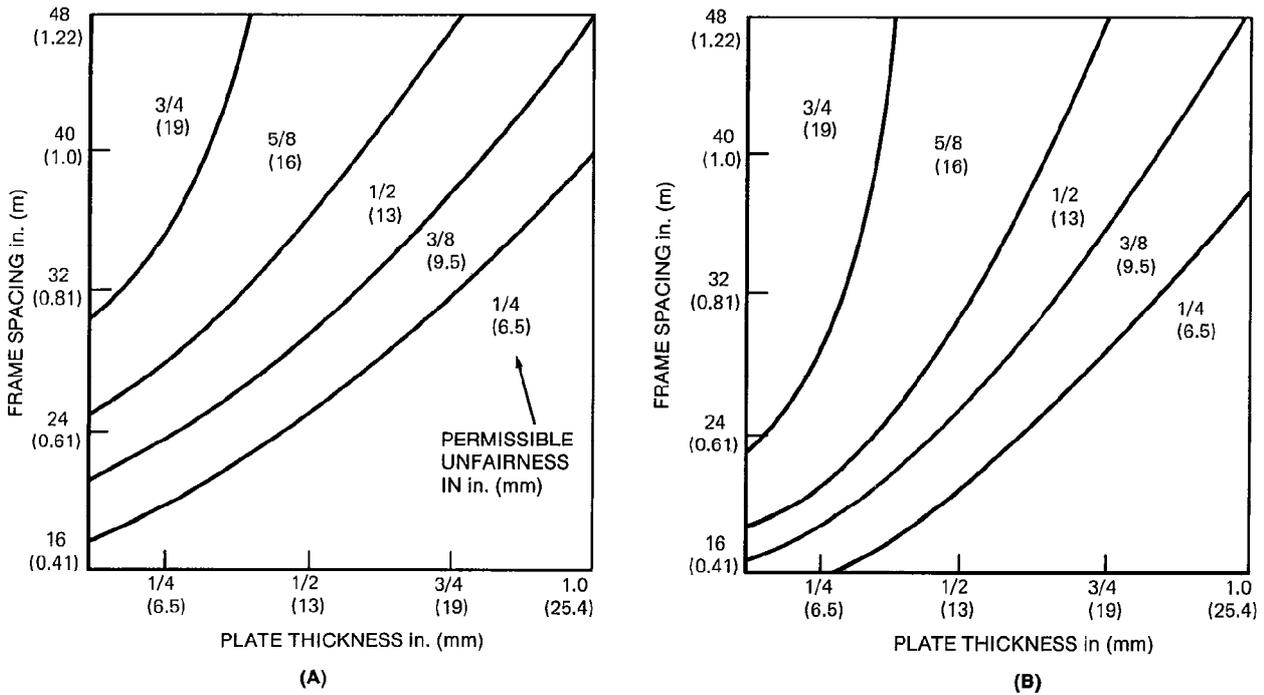
**Figure 45—Permissible Unfairness in Steel Welded Structures as Used for Guidance by U.S. Navy**
