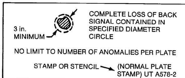
**Figure D-10—A578 Minimum Acceptance Criteria and Marking Requirement**
