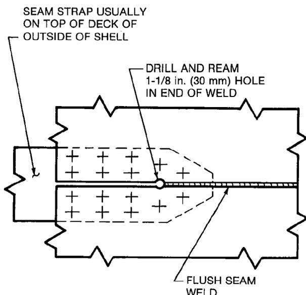
**Figure 23—Transition From Riveting to Welding in Flush Seam**
