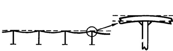
Figure 42—Angular Deflection Due to Welding Stiffeners to Plate (The Washboard Effect)
