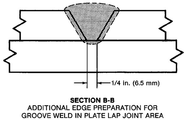
**Figure 22—Two Methods of Edge Preparation for Groove Welds Near Plate Laps**
