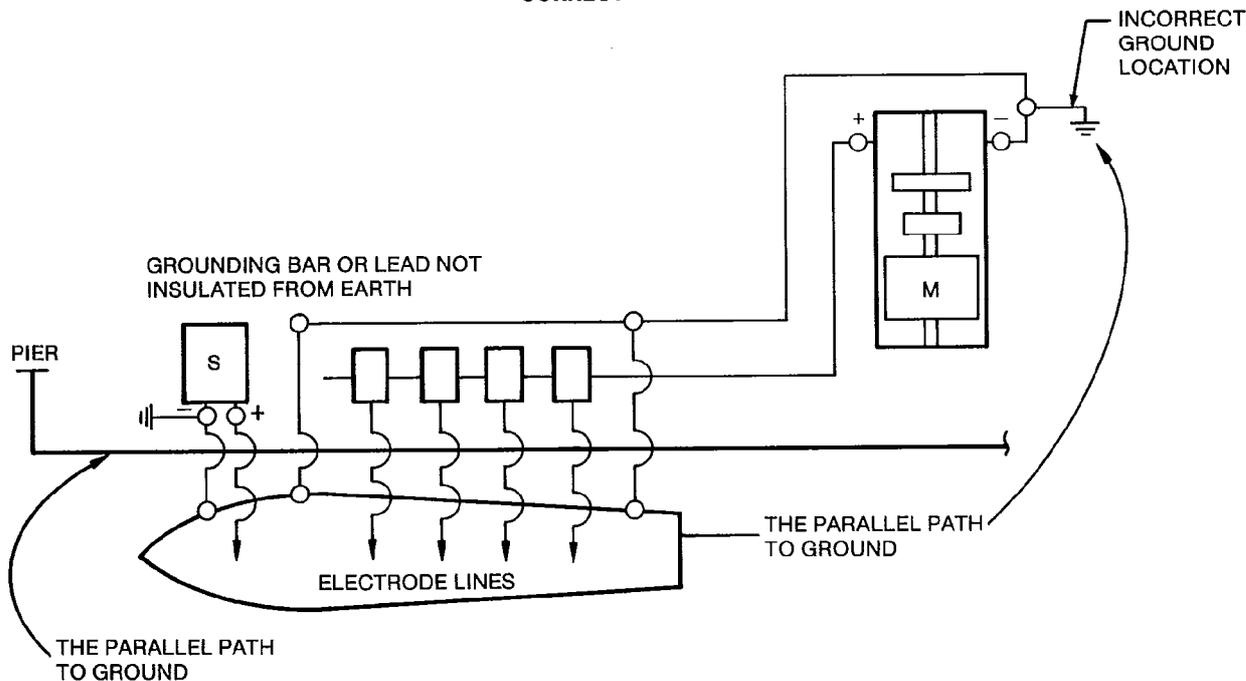
NOTE: WITH NEGATIVE SIDE OF GENERATOR OR RECTIFIER GROUNDED, PART OF THE WELDING CURRENT FLOWS FROM THE SHIP'S HULL TO THE WATER AND EVENTUALLY REACHES THE NEGATIVE SIDE OF THE GENERATOR OR RECTIFIER.
