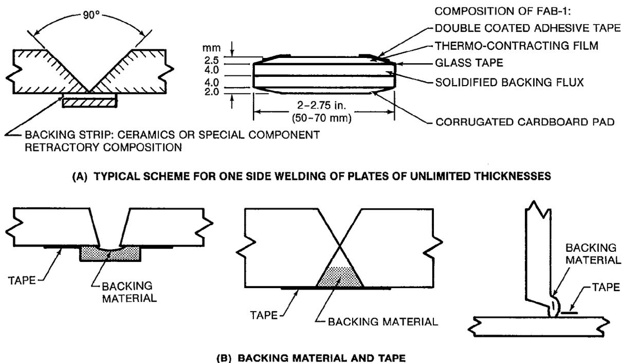
Figure 11—Typical Joint Details for One-Side Welding
