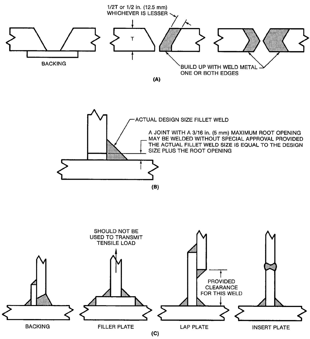
Figure 31—Correction of Poor Fit-Up
