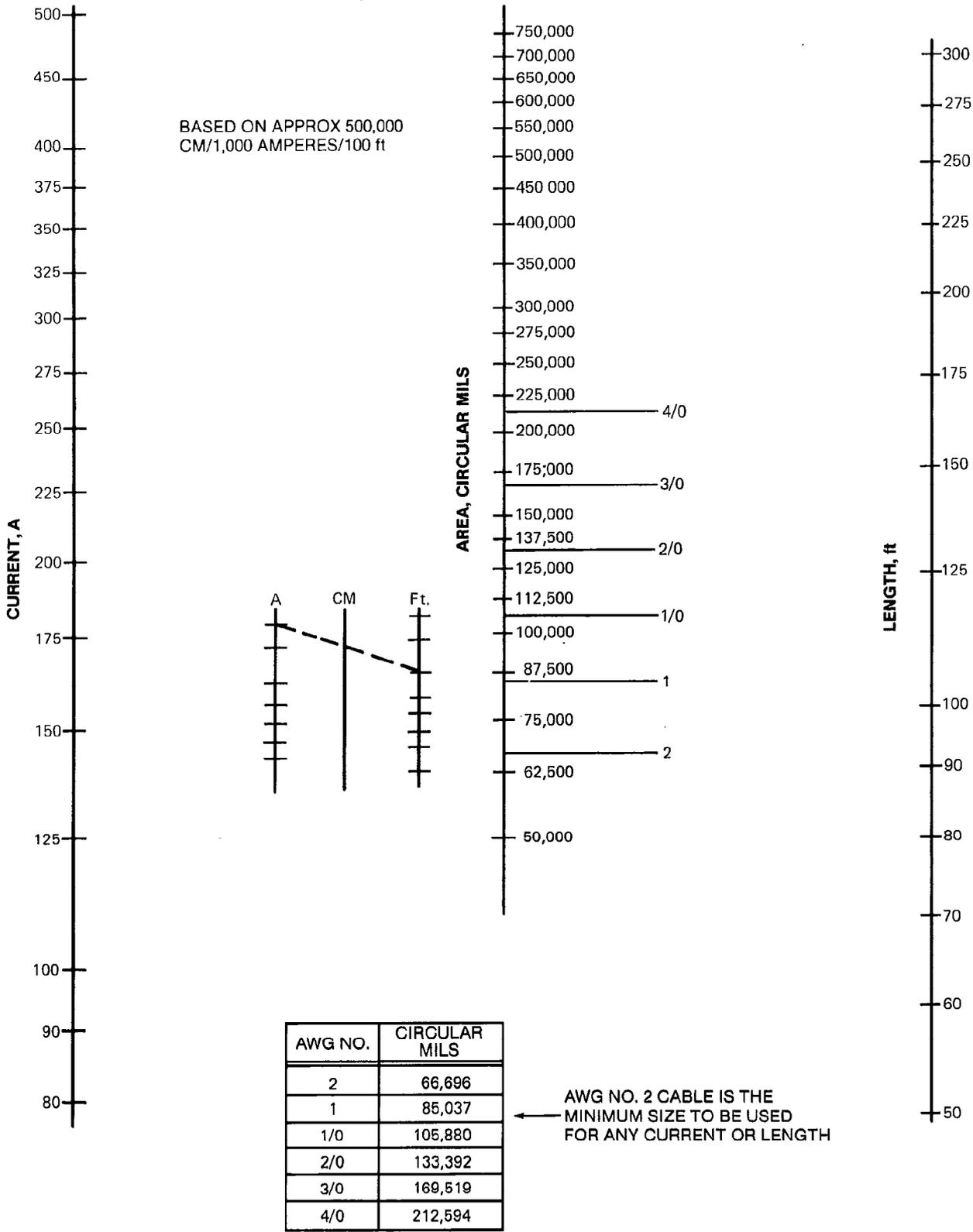
Figure 55—Nomograph for Copper Electrode Lead Cable Size
