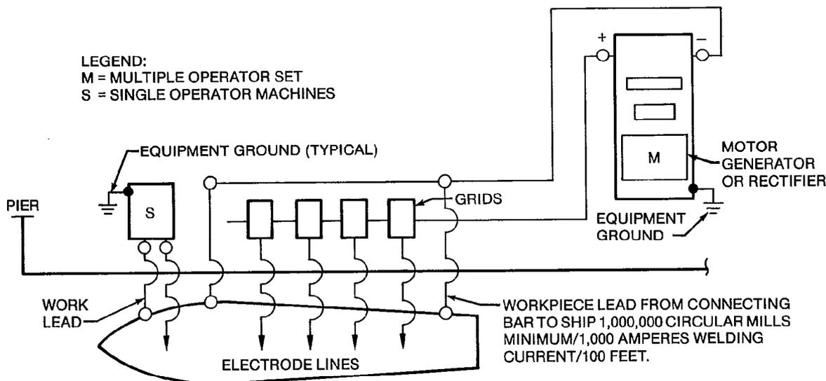
NOTE: CONNECTING BAR OR LEAD SHALL BE INSULATED FROM EARTH, CASE OF MACHINE, AND OTHER STRUCTURES, BE OF SUFFICIENT CROSS-SECTIONAL AREA TO CARRY THE WELDING CURRENT, AND SHOULD REMAIN ABOVE WATER WITH TIDE CHANGES OR SHIP MOVEMENTS.
