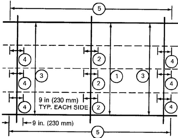
1. Panels 1 and 2 are complete with internals welded to within 9 in. (230 mm) of edges of panel.
