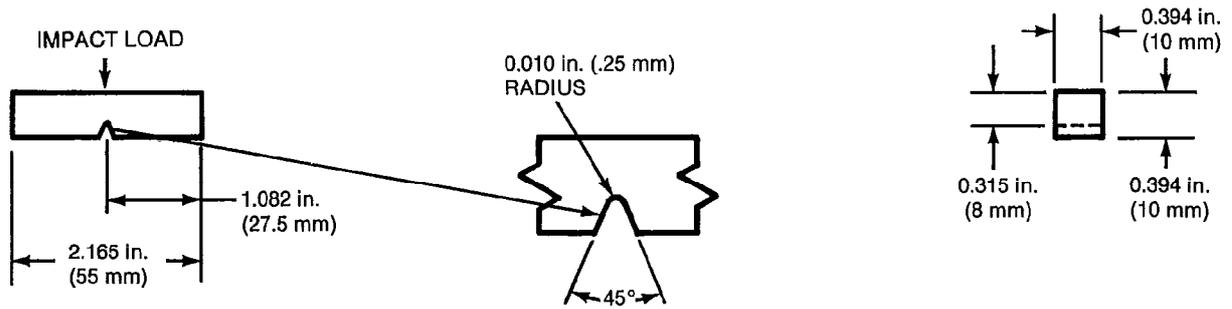
**Figure 2A—Standard Charpy V-Notch Test Specimen**
