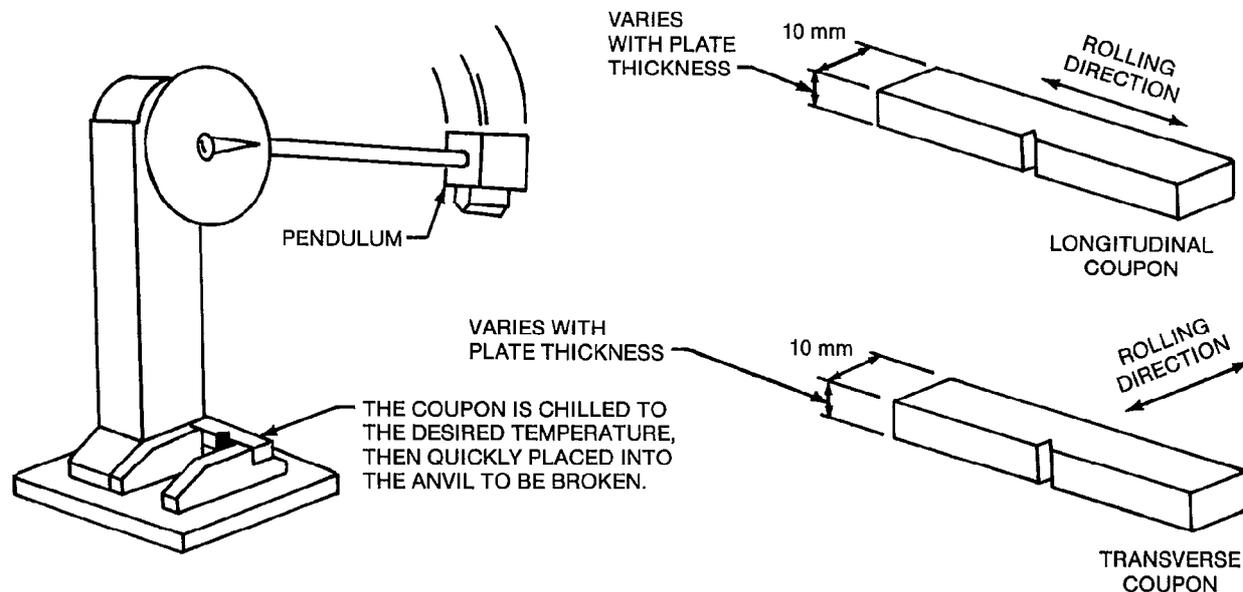
Figure D-5—Charpy Coupon Testing
