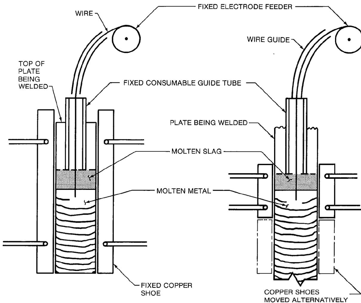
Figure 10—Consumable Guide Tube Welding
