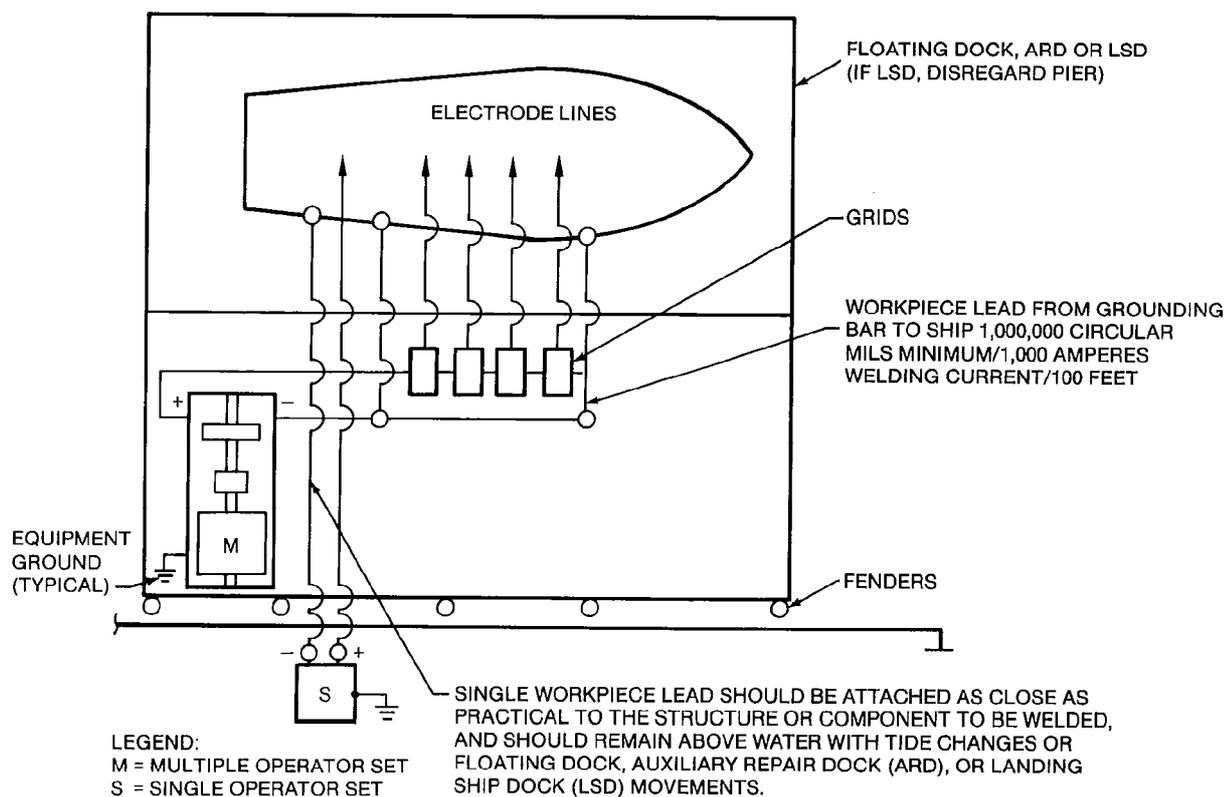
NOTE: CONNECTING BAR OR LEAD SHALL BE INSULATED FROM EARTH, CASE OF MACHINE, AND OTHER STRUCTURES, AND BE OF SUFFICIENT CROSS-SECTIONAL AREA TO CARRY THE WELDING CURRENT.
