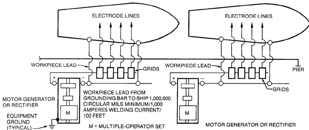
NOTE: WELDING ON TWO OR MORE SHIPS (IN CASE OF MULTIPLE-OPERATOR MACHINE) SHOULD NOT BE PERFORMED WITH THE SAME GENERATOR OR RECTIFIER.
