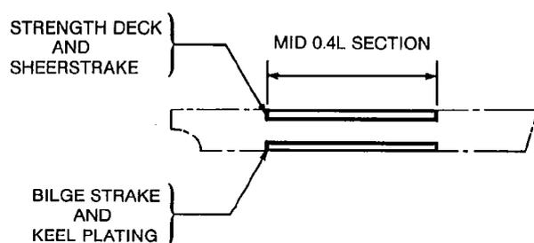
**Figure 12—Most Highly Stressed Areas of Hull Girder**
