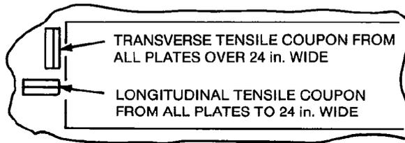
Figure D-2—Tensile Coupon Sampling
