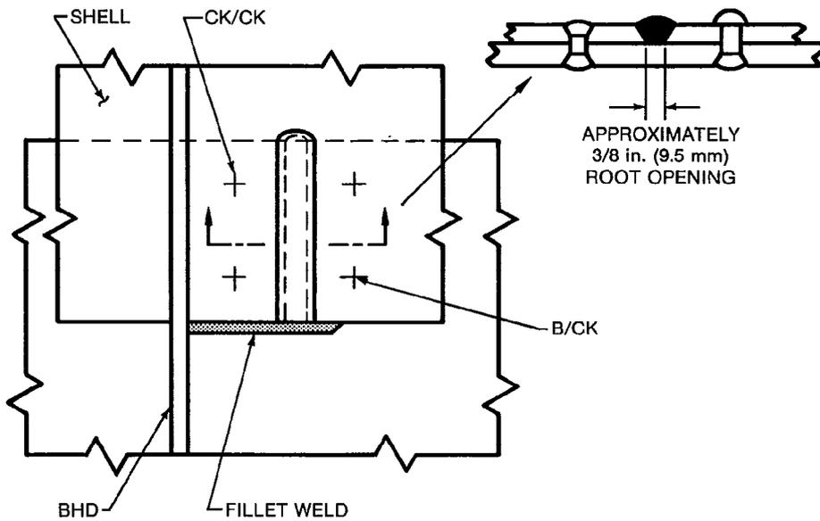
Figure 26—Welded Stops at Riveted Seam Lap
